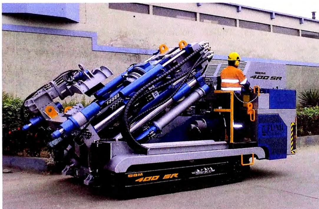
**Fig. 1.2** Máquina perforadora Raise Borer, modelo SBM 400 SR.
