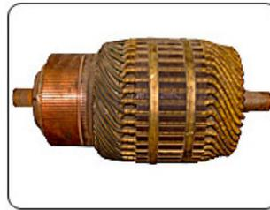
Armature with steel binding wire
