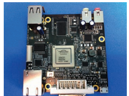
▲ PCB copper traces for the PCoIP zero client modeled in ANSYS Icepak shows the substrate with die as a heat source, two DRAM devices, a flash device and an audio codec device.
