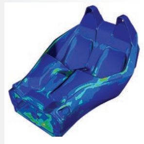
▲ Evaluating failure criteria for all layers in the monocoque saved time and money.
