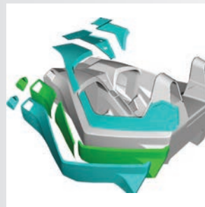
▲ The composite monocoque exterior shell has more than 300 pre-cut layers.
