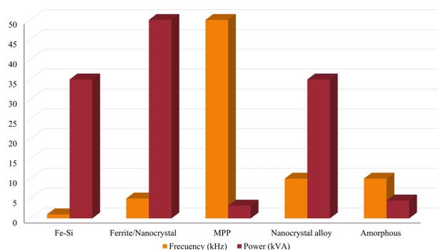
FIGURE 6. Magnetic materials comparative used in transformers.
