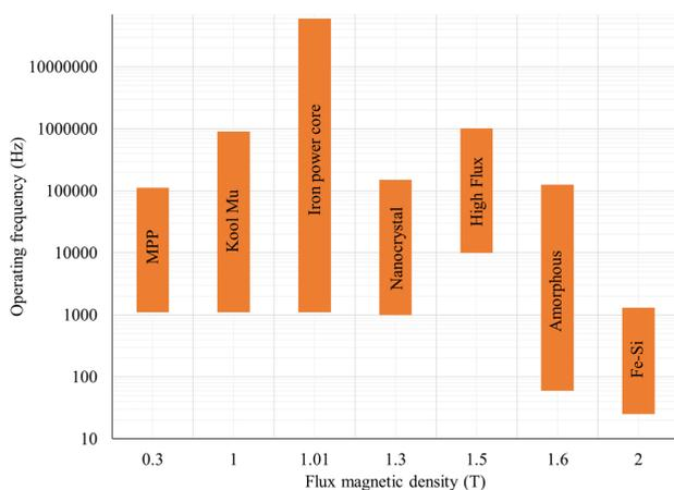
FIGURE 4. Magnetic materials' operating frequency and magnetic flux density.
