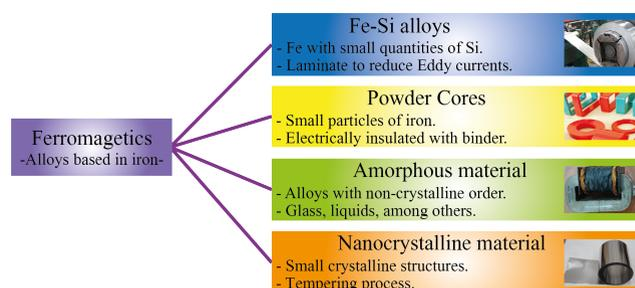
FIGURE 1. Magnetic materials used in PECs cores.
